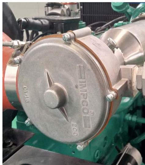
The proportioning mixer of IMPCO company is used in fuel control and air-fuel mixer.
